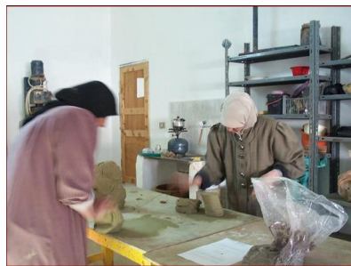
Figure (22): Slurry Partial Drying, Wedging and Kneading.
