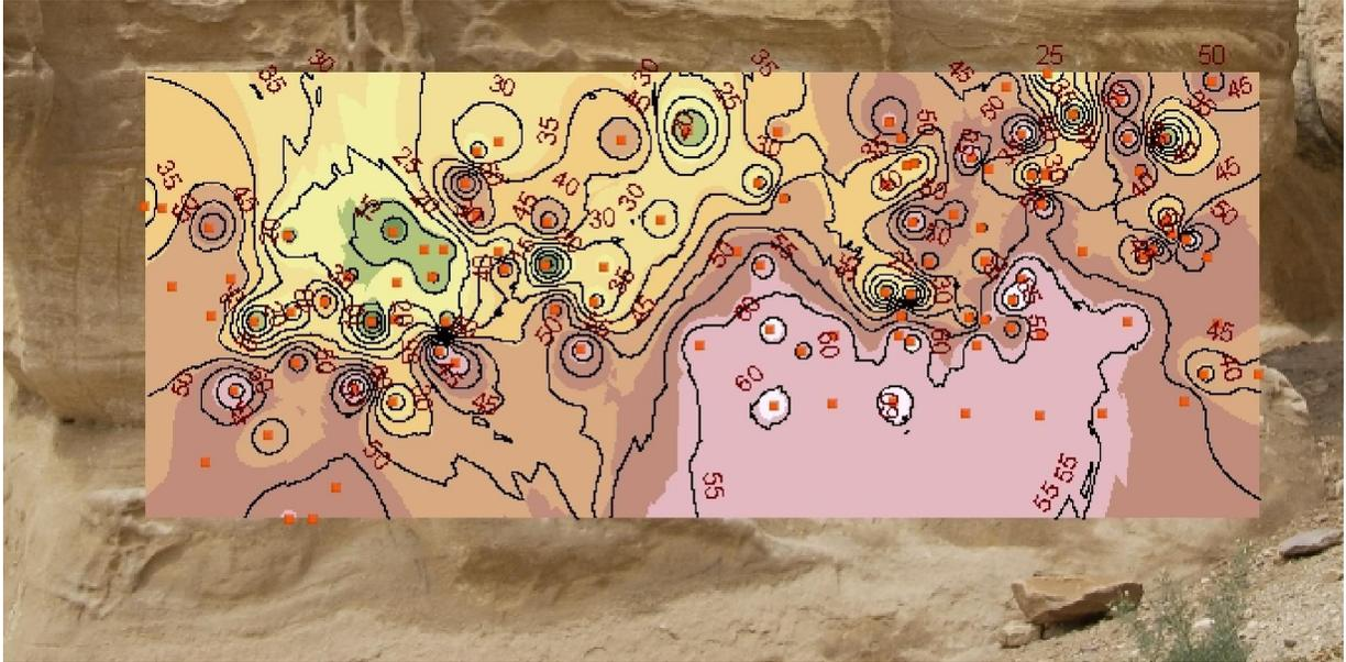
**Figure 8: Calcium Grid Distribution and Contours (Contour labels are in %)**
