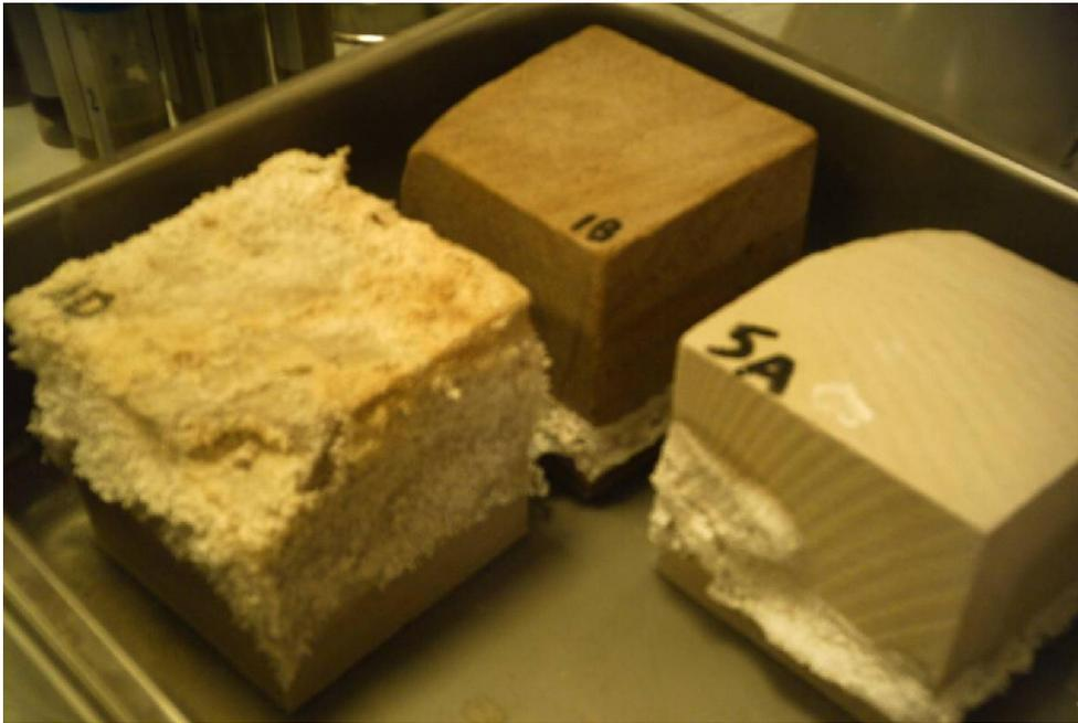
**Figure 15: The salt test after 20 days. 1D on the left was untreated. 5A was treated with funcosil100, while 1B was treated with Funcosil 300. The latter seems to yield better protection against salt rise. In the following pictures the stone samples are also shown individually and from the top.**
