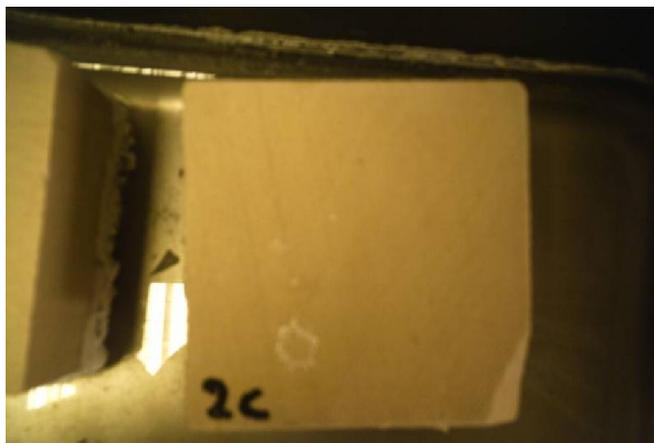
**Figure 16: Stone samples and the salt test shown individually (2c is for tetraethosxy silane)**
